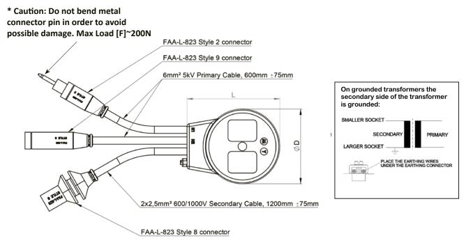
Notice: If transformer is equipted with earthing connector it has to be allways grounded by connecting it using continuity wire/conductor etc. into ground potential
